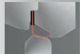
Tight sealing up to max. +260°C with metallic sealing ring
