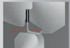
Minimized friction via reduced contact pressure of the disc and the metallic sealing ring
