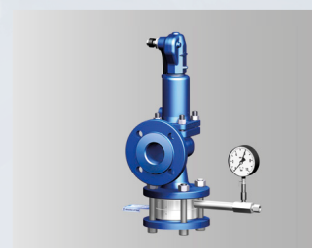
SAFE Combi-R – zero leakage allows the use of certain types of media which tend to harden or become sticky when in contact with the atmosphere. Protects the safety valve against corrosion.
